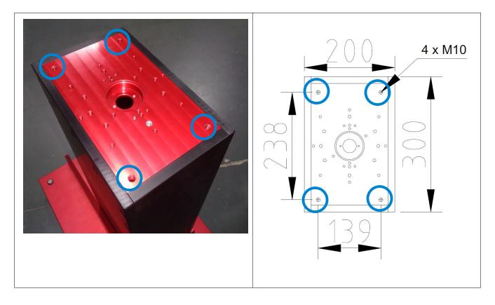
Once the mount will be placed on the pier, it must be fixed on this support matching the four fixing screw slots on the corresponding hole threads.
