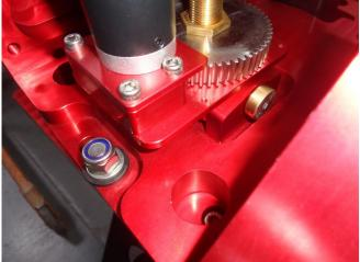
One of the four fixing holes, the one shown in the picture on the right, is partially covered by a gear carter, that need to be removed to clearly see the hole slot and screw the fixing bolt.
