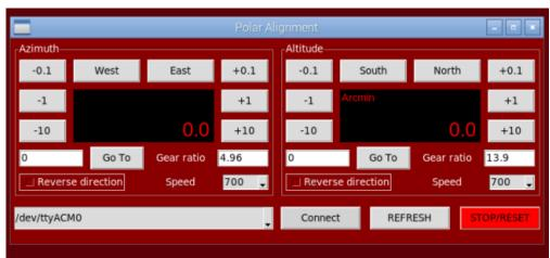
In order to start the motors managment, click on the connect button, when it will turn green and the label change from connect to disconnect, the connection will be established.
