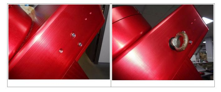
The lift eyes can be used to attach lifter hangers and lift up the mount, in order to place it on the Pier.
