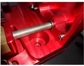
When all the four bolts will be screwed on their corresponding holes, it will be possible to mount again the gear carter and to assemble the Motorized Polar Alignment System controller.
