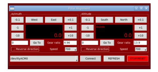
In order to start the motors managment, click on the connect button, when it will turn green and the label change from connect to disconnect, the connection will be established.
