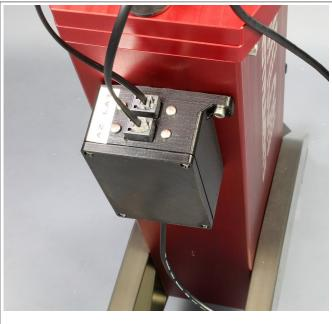
The Motorized Polar Alignment kit controller must be powered with it's dedicated 12V power supply provided in the package and connected via USB to one of the StarGo2 Pro USB ports available.
