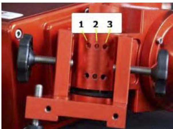
5) Screw the brass item in position 1 for latitudes from 10^{\circ} to 40^{\circ} or in position 3 for latitudes from 45^{\circ} to 70^{\circ}
