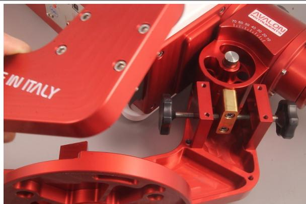
Unscrews the two screws and remove the brass latitude adjustment plug.
