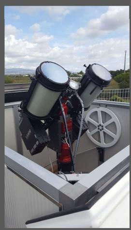
Two channel spectropolarimeter based on Magneto Optical filters for the simultaneusly production of magnetograms and doppelrgrams at high cadence and high space resolution.
