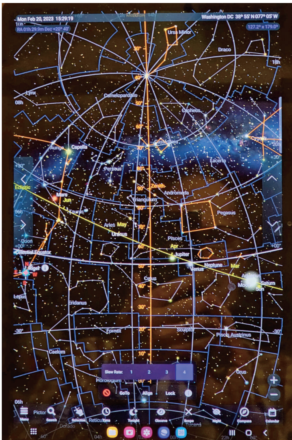
Figure 7. Sky Safari 7 Pro display connected to StarGo through Bluetooth. Note sky position of mount shown at left below Celestial Equator, near Rigel. Slew rate is shown in the purple boxes near bottom.
