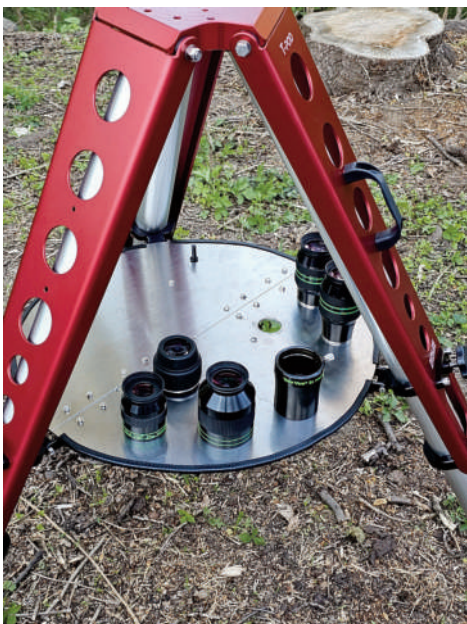
Figure 4. Circular plate (fabricated by owner) for eyepieces and other gear
