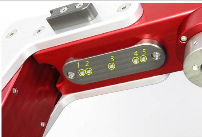
Assemble the counterweight shaft on the counterweight fixing plate on the bottom of the DEC arm by screwing the small screw in one of the three treated holes available. There are five available position to fix the counterweight shaft, depending on the setup. It is also possible to assemble two counterweight shafts.
