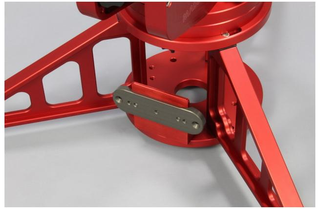
At this point it is possible to adapt the StarGo box directly on the pier.
