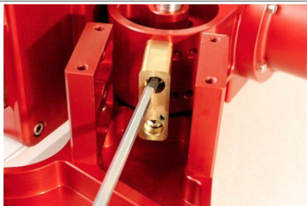
Place the brass latitude adjustment plug over the set of holes (1, 2 or 3) corresponding to the needed latitude range as described on the previous page. Re-attach the brass plug in the preferred latitude range position using the screws removed earlier. The mount is shipped from the factory with the brass post in position 2.
