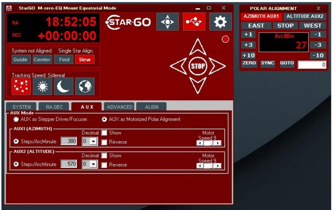
**This tool allow to move the selected motor with the ArcMin unit, allowing also to perform GoTo by simply typing the choosen value in ArcMin and pressing on the GOTO button.**
